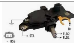
Regulador Tipo BOSCH F00M144131/185/186 F00M145301/303/321/858 RENAULT CLIO 1.2 - MEGANE 1.6
